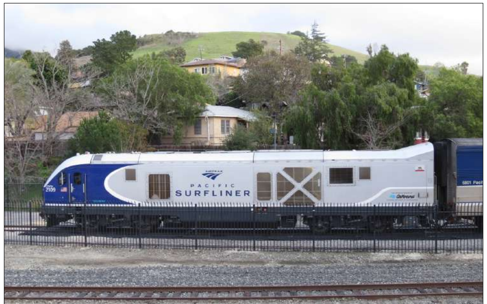
Long, lean, and quiet. New Charger locomotives began appearing with the midday Surfliner to and from San Luis Obispo near the end of 2018. Unlike previous Amtrak/Caltrans locomotives produced by General Motors and by General Electric, these come from the Germany-based Siemens' factory in Sacramento, and use alternating-current rather than direct-current traction motors.
