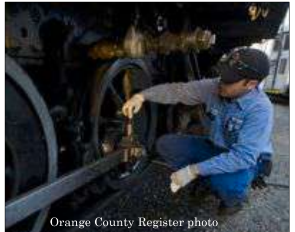
Lubrication cups atop bearings used wicks, drips, or pressure to deliver oil or grease. Orange County Register photo
